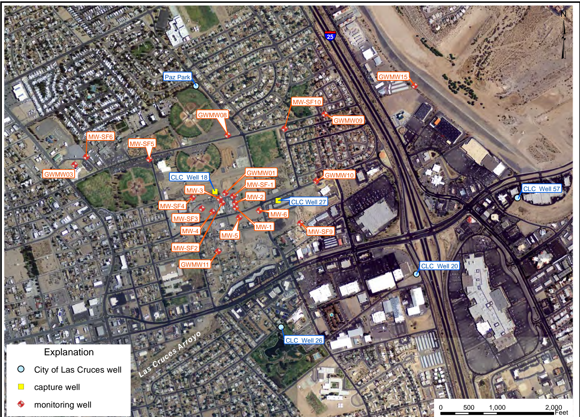
Figure 1. Aerial photograph of the Griggs and Walnut plume site showing locations of capture wells and monitoring well network, City of Las Cruces, New Mexico.
